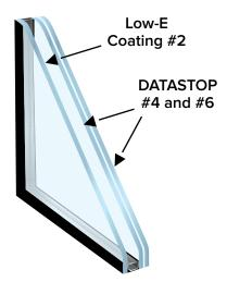
This 1-5/16" configuration increases attenuation, thus providing a higher level of electronic eavesdropping protection than CyberShield alone.
